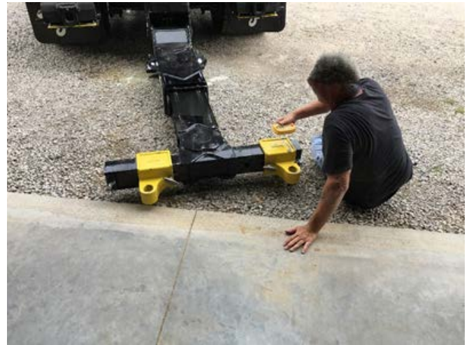
Photo 5. Use of remote to position lift forks
