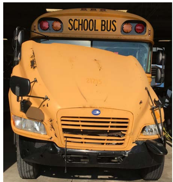
Photo 11. Damage to front of school bus
