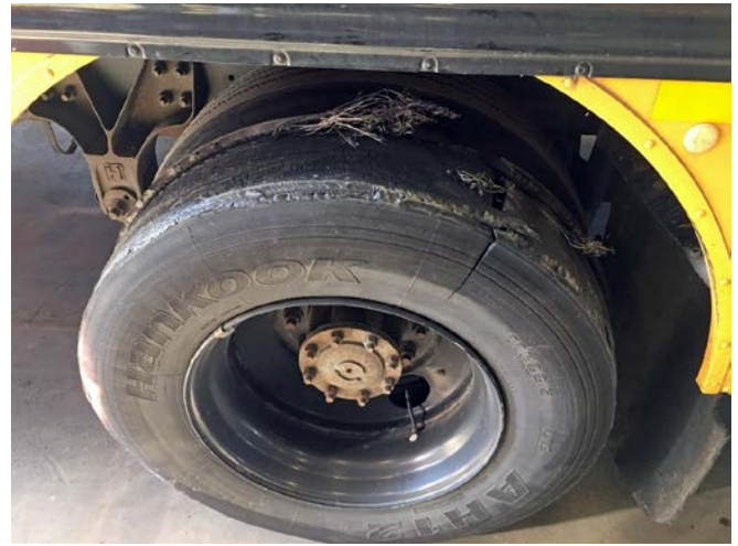
Photo 4. Driver's side outside dual rear tire of school bus causing driver to exit expressway
