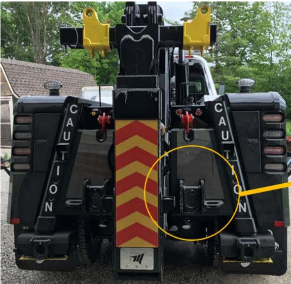
Photo 8. Yellow paint transfer from school bus on rear of tow truck
