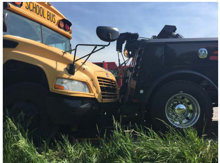
Photo 7. Front of school bus pushed 10-12 feet forward into rear of tow truck.
