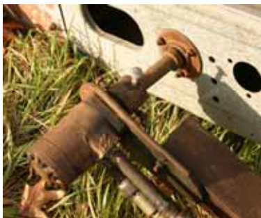
A farmer died when his clothing became entangled in an unguarded rotating motor drive-shaft on a farm-modified ear-corn elevator. MIFACE Investigation Report 08MI135
