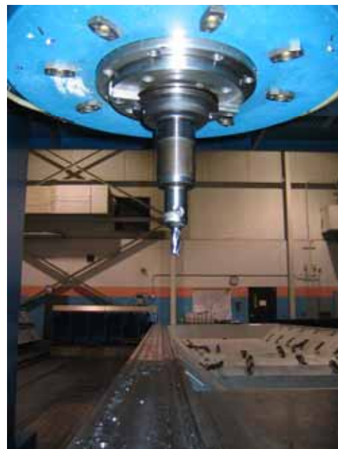
A male machinist died when he contacted and then his clothing became entangled in the rotating vertical cutting head of a gantry mill.
