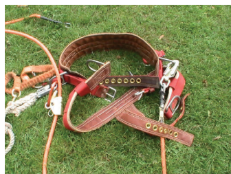
Tree trimmer died due to a 40-foot fall when the top of the elm tree to which he was tied off broke away from the tree after the tree trunk was struck by a swinging tree branch.
