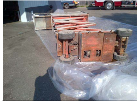
Case 19. Male painter died when the tire of the elevated Skyjack 3220 scissor lift in which he was working entered a depression in a parking lot caused by a recessed storm drain and tipped to its side.
