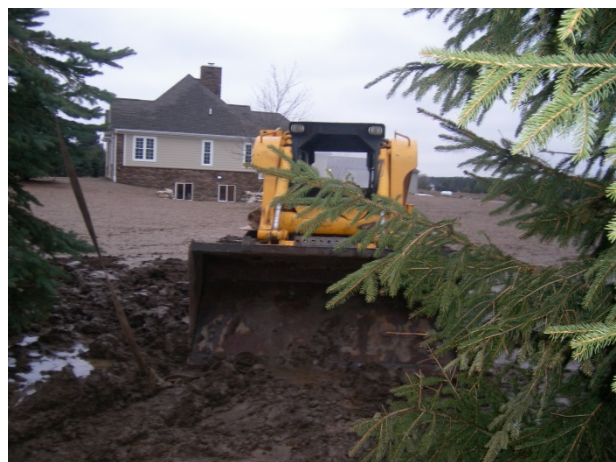
Case 55 . Male landscaping business owner crushed between the lift bucket arms connecting the cross member and the front frame of a Gehl Model 7800 skid steer loader.
