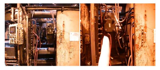
Figure 9. Pictures of the aluminum die cast machine with a cold chamber
