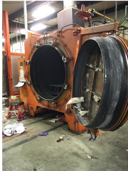
A maintenance worker in a manufacturing plant died when struck by part of a pressurized stainless-steel furnace door that ruptured. Narrative #58
