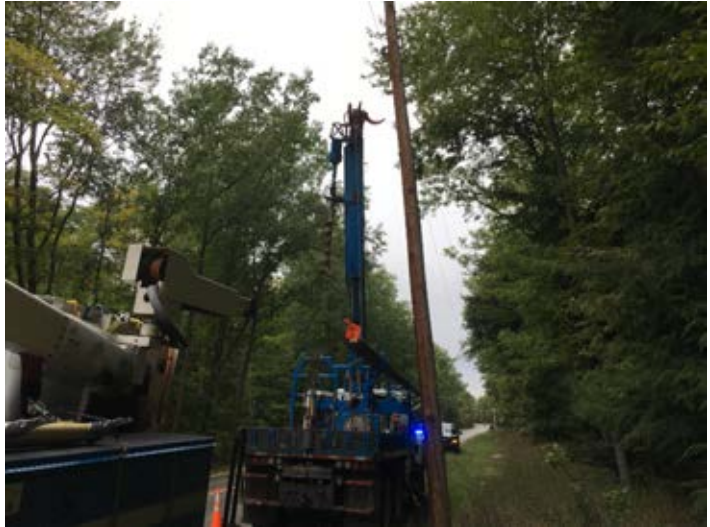
A journeyman lineman in his 50s was electrocuted when the boom of a digger derrick contacted an energized 7200-volt power line.
