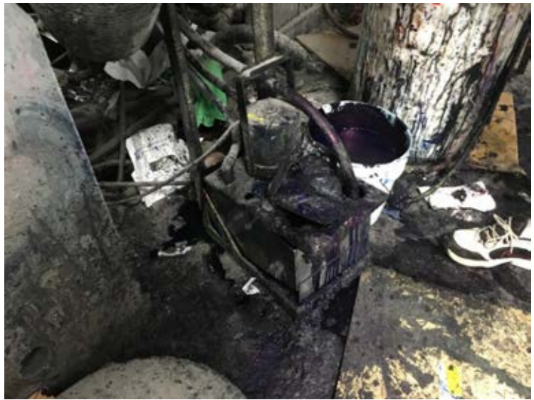
A male machine adjuster in his 40s died when he contacted the upper frame of a pump that was energized by a damaged cord and plug.
