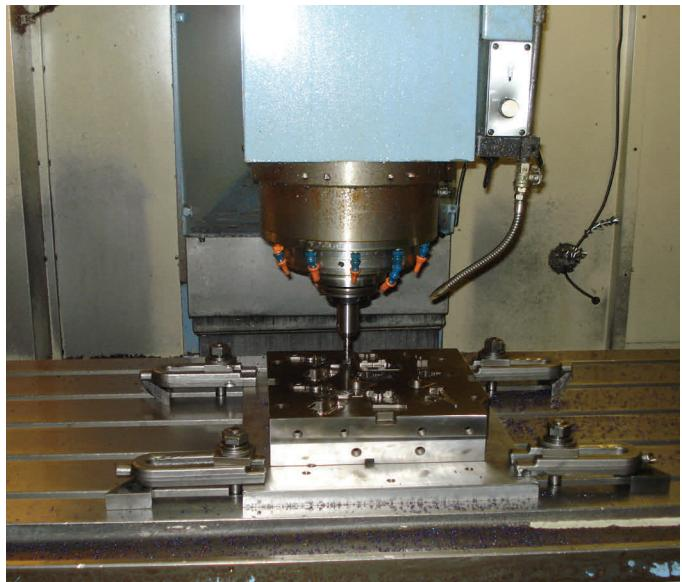
This picture shows metal being machined to manufacture a mold to be used in plastic injection. MWFs were sprayed on the metal being machined. The MWF runoff and metal shavings were collected in a large container located under the machine.
